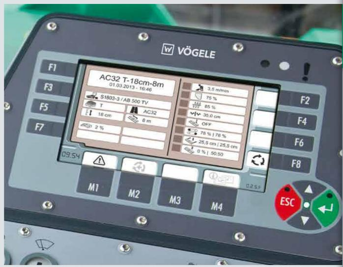
The automatic Paving Programs function allows the operating personnel to store their own paving programs. All key parameters for paving a specific layer (example: base course of asphaltic concrete, 18cm thick) can thus be saved.
