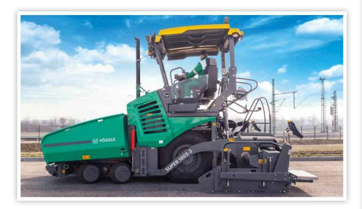
**The SUPER 1803-3** combines at a high level of perfection features such as sturdy and reliable material handling, large pave widths up to 8m and extremly high mobility.
